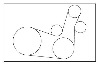
The engine drive belt on this hybrid vehicle is under a higher tension than the engine drive belt on a non-hybrid vehicle and requires the use of a special kind of tool to service. See your dealer/retailer for service.
